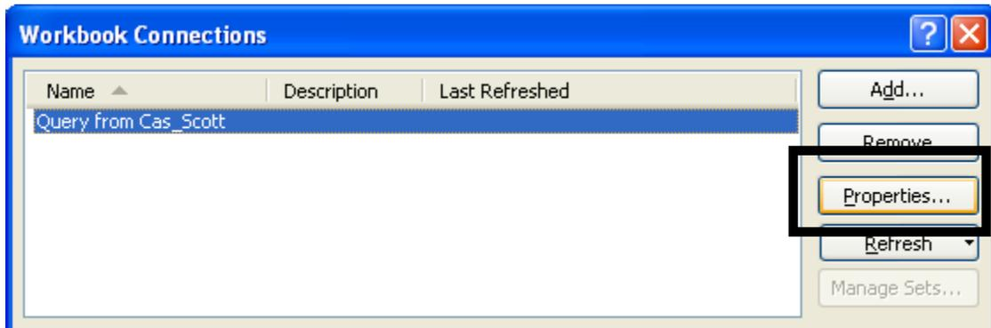
On The Usage Tab of the Connections Properties box, Select "Refresh Data When Opening File"
